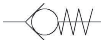
Rückschlagklappe federbelastet (Option) Spring-actuated swing check valve (optional)
